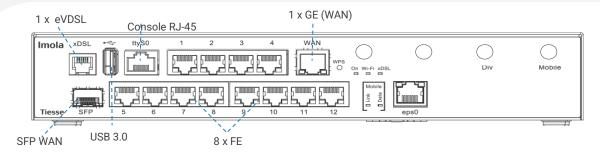
The Imola x872 series is an innovative line of routers with VDSL Enhanced ultra broadband and fiber connectivity, with 14 Ethernet ports (5 Gigabit and 9 Fast Ethernet) and Wi-Fi.
