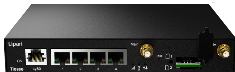
Lipari 5200-IKW with the SIM flap opened
