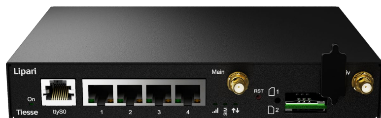
Lipari 5200 with the SIM flap opened
